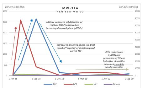
Results show single injection event produced influence > 100ft downgradient MW-32A (76.1% reduction [TCE] MW-29) Minimal additive based carbon present yet sustainable *and* complete biotransformation within biostimulated ecosystem. Visit our website to read more about how you can realize <u>cost-effective</u> and *complete* chlorinated remediation success.
